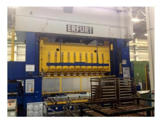
The **ERFURT PTRZSST 210 mechanical transfer press** was produced in Germany in 1991. The machine has a pressing force of 160 tons. The upper table is capable of 20-40 strokes per minute with a maximum size of 400 mm. The press is equipped with ten stands.
